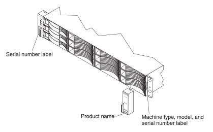
Figure 63. Serial number location on the DS3200
